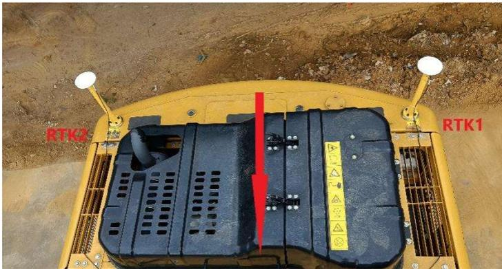
5. The 4G sucker antenna should be arranged according to the on-site location as required below: (1) The magnet adsorption is available at the arrangement location; (2) The signal is unobstructed.
